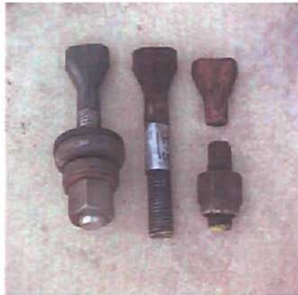
Figure 1-3 1½” Mill Liner Bolts (Broken Bolt On Right)
