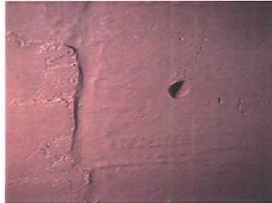
Figure 1-4 Racing Damage (Left of Liner Bolt Hole)
