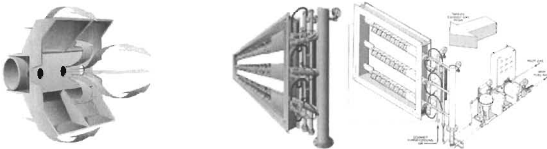
Figure 20 – Individual Burner and Array within Supplementary-Fired HRSG (Coen)
