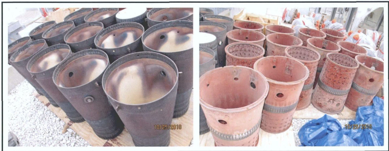
Figure 5. Replacement Combustor Liners and Flow Sleeves (14 Sets/CT) Planned for Unit 8.
