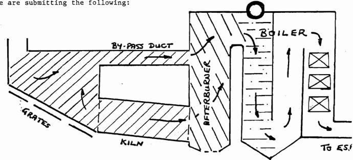
Zone 1 - Furnace, Rotary Kiln and By-Pass Ducting
