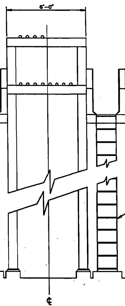
TYPICAL PIPE SUPPORT OVER ROADWAYS, RAILROADS AND BUILDINGS.
