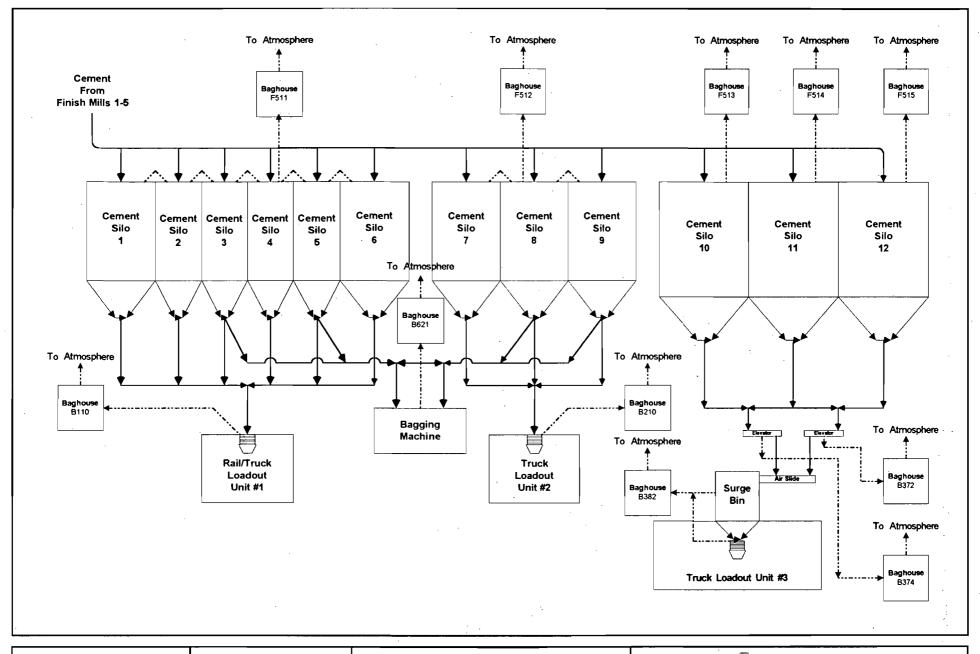
Attachment TA-E12-L1 Process Flow Diagram Tarmac America Medley, FL
