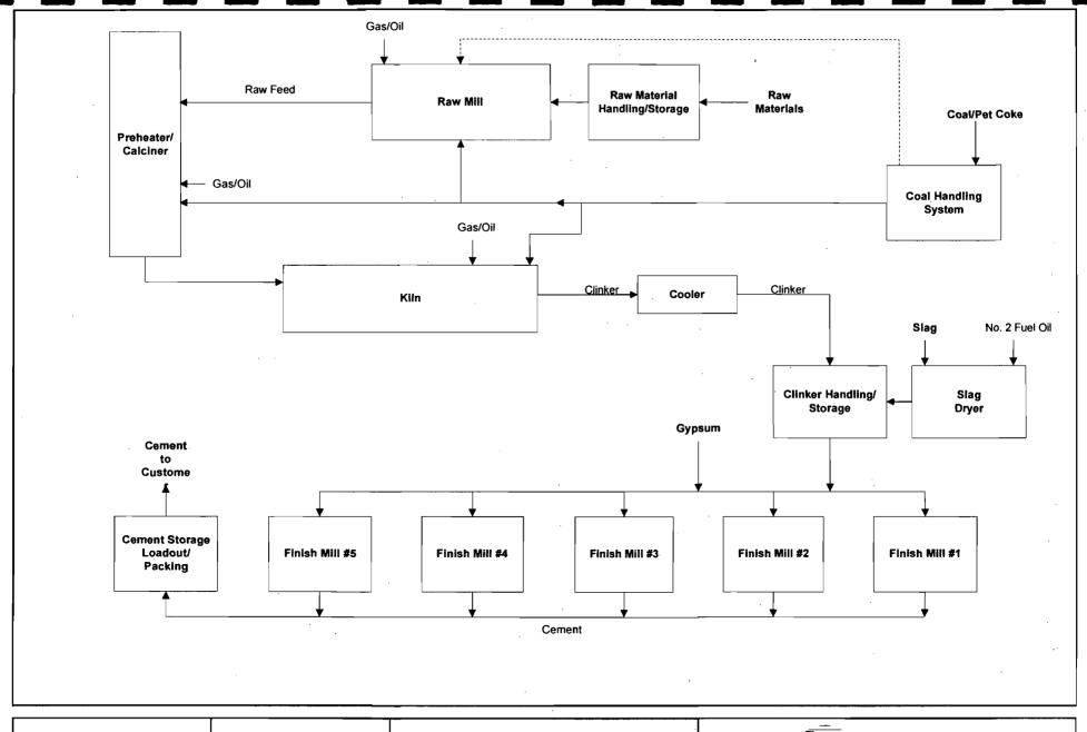
Attachment TA-FE-E1 Process Flow Diagram Tarmac America Medley, FL
