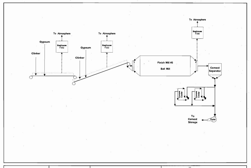
AttachmentTA-E03-L1 Process Flow Diagram Tarmac America Medley, FL
