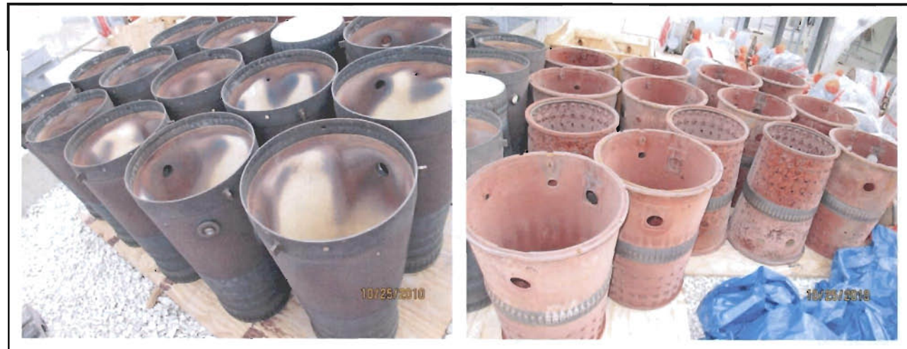
Figure 5. Replacement Combustor Liners and Flow Sleeves (14 Sets/CT) Planned for Units 4 and 5.
