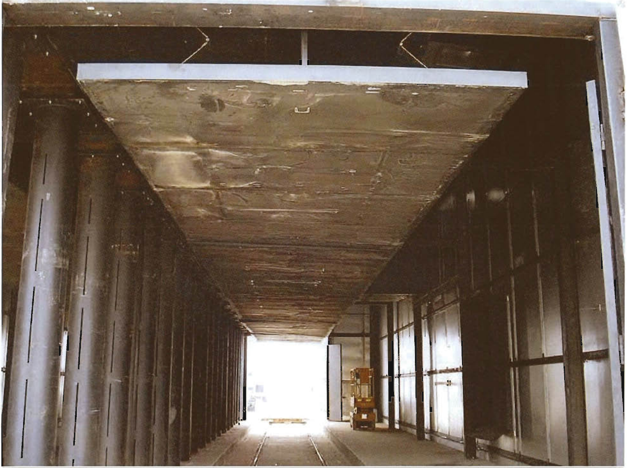
PNEUMATIC OVERHEAD BAFFLES KEEP TOP LAYERS FLAT AND HAS SHOWN IMPROVEMENTS OF 1% TO 2% IN 2 & BTR
