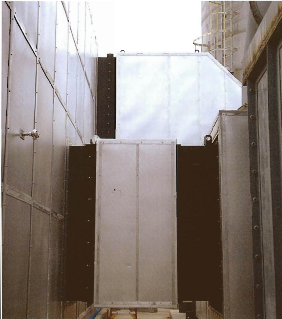
KDS KILN SIDEWALL WITH TIE BARS ASSURING FLAT PERMANENTLY SECURE PANELS
