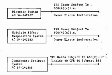
Pursuant to 660(2)(a) And 40 CFR 60.283(a)(1)(iii), Owner Elects To Combust Gases From NSPS Stripper With Other Waste Gases In Incinerator Or Other Device, Or In Lime Kiln Or Recovery Furnace Not Subject To NSPS And Subjection To 1200°F For 0.5 Second. NOTE: This Option Available Only Because Gases From NSPS Sources Are To Be Combined With Those From Non-NSPS Sources. Reason For This Exception—Section 111 Of The CAA Only Authorizes EPA To Promulgate Emission Standards For New Sources.
