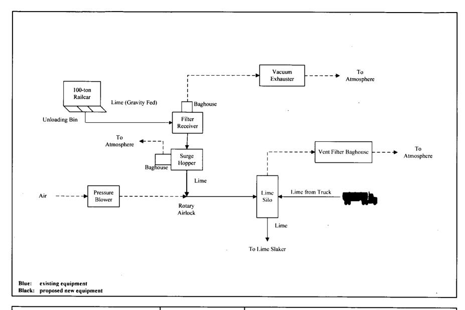
Attachment IC-EU1-I1 Lime Handling System Process Flow Diagram Indiantown Cogeneration, L.P. Indiantown, Florida
