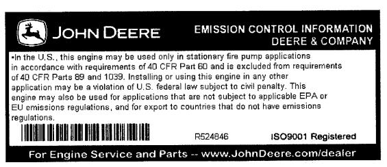
This label applies to all of the following engine models, sold to Clarke Fire Protection, for use in stationary fire pump applications:
