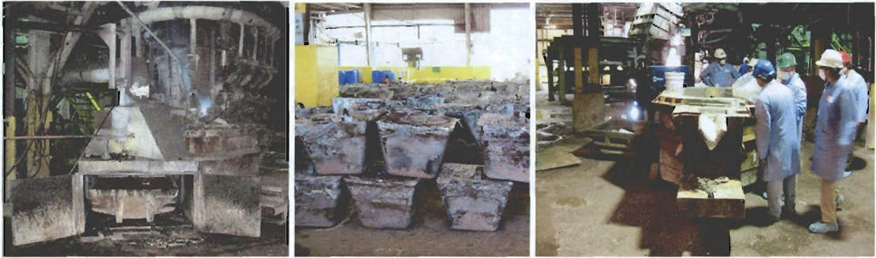
Figure 10. Blast furnace tapping, 2-ton buttons, holding kettle can be moved to refining area.
