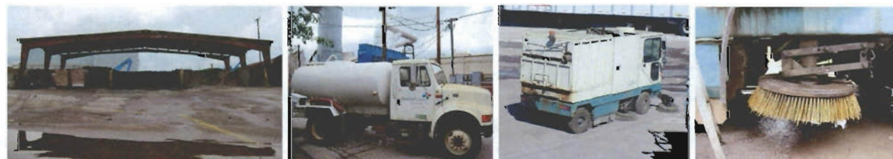
Figure 14. Storage area and wetted pavement, watering truck, wet sweeper truck, wet brush.
