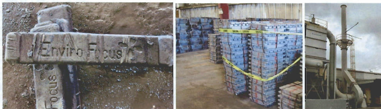
Figure 13. Individual ingots, stacks of ingots and larger blocks, refining baghouse and stack.
