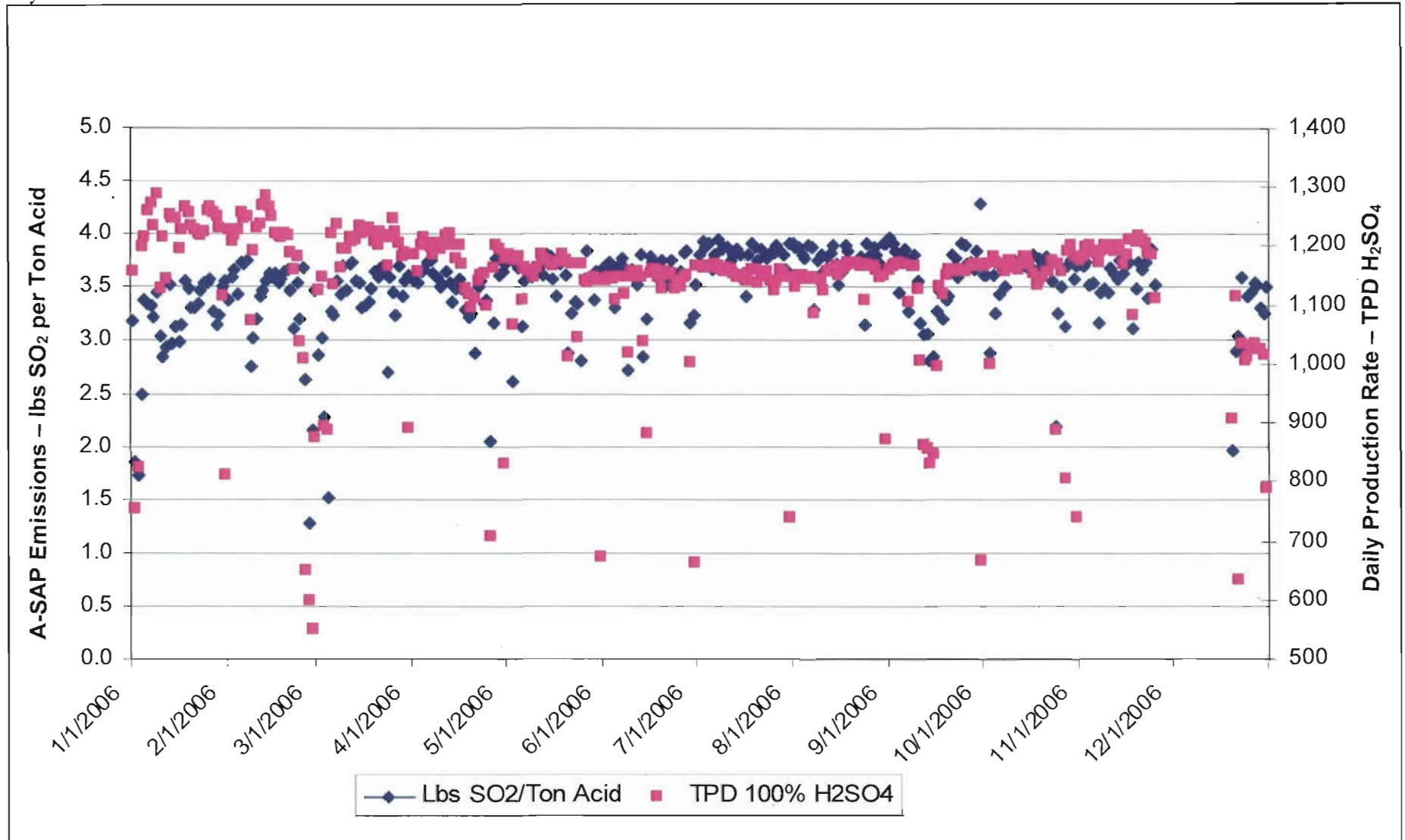
Figure B-1 CF Plant City Phosphate Complex A-SAP SO 2 Emissions - Daily Average Pounds SO 2 /Ton H 2 SO 4
