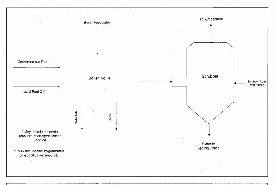
Attachment USS-EU1-I1 Process Flow Diagram U.S. Sugar Corporation Boiler No. 4
