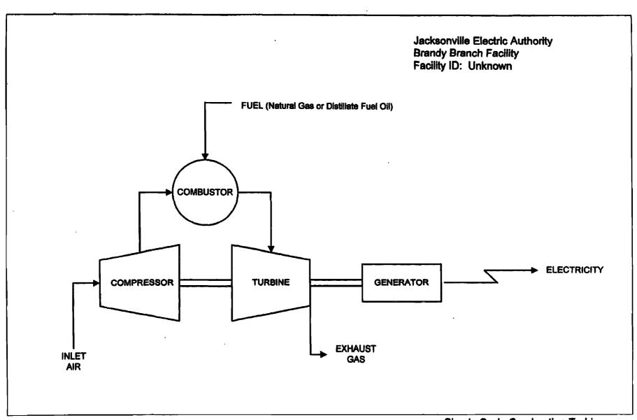
Simple Cycle Combustion Turbine Process Flow Diagram
