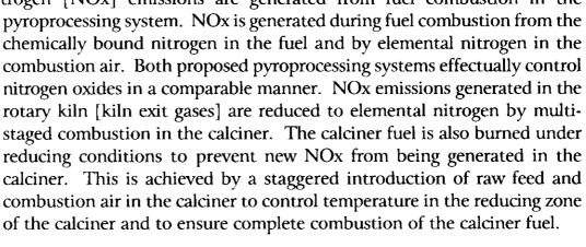
Through these process mechanisms both fuel NOx and thermal NOx will be controlled to meet the revised NOx emission limits requested in the construction permit revision. Again, both equipment manufacturers have guaranteed the requested emission factor, and the use of the CEM system conditioned in the existing permit will ensure that the described process control will be effective.
