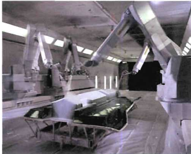
Figure 5. Robotic Application of Gel Coat
