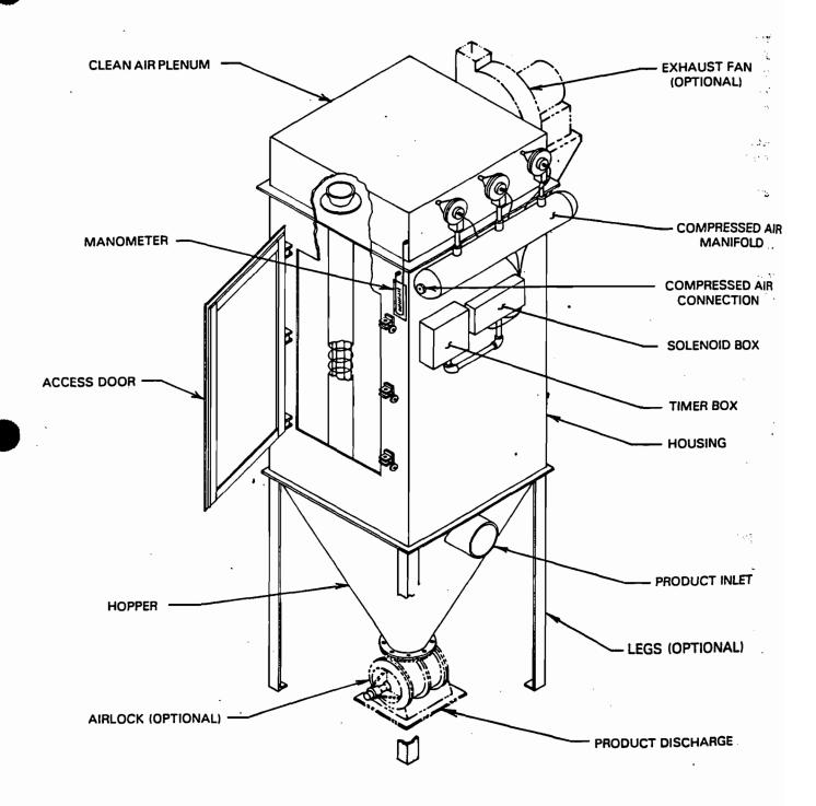
Figure 1 — Super Jet Filter Assembly
