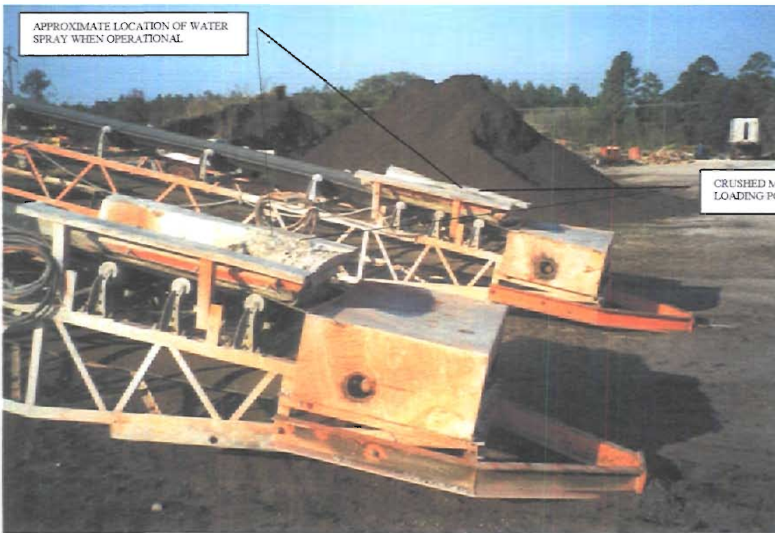
CLOSE-UP VIEW OF LOADING POINT AND WATER SPRAY AREAS ON CONVEYORS.
