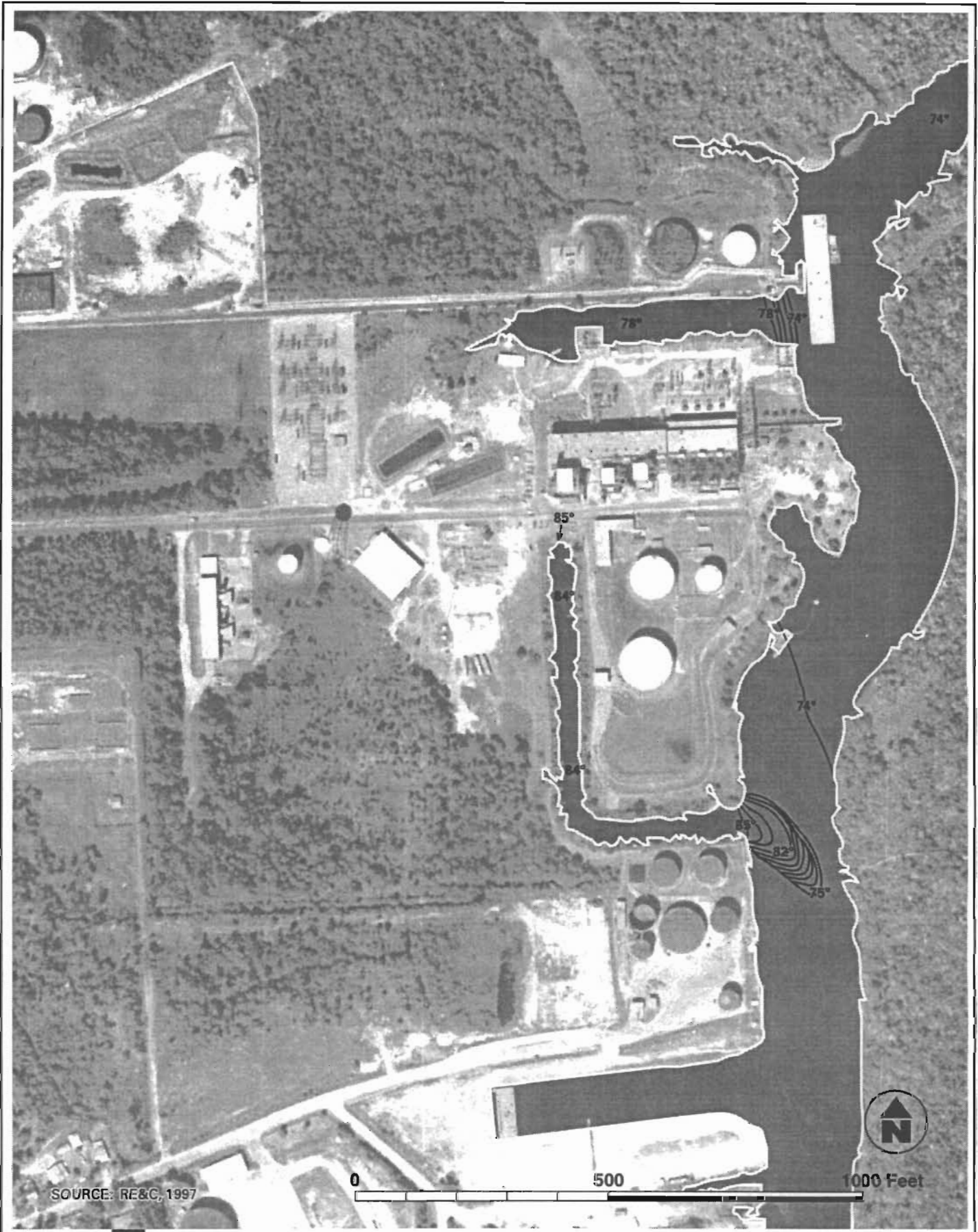
THERMAL PLUME FOR UNIT 7 ONLY OPERATIVE PURDOM UNIT 8 PROJECT - ST MARKS FLORIDA
