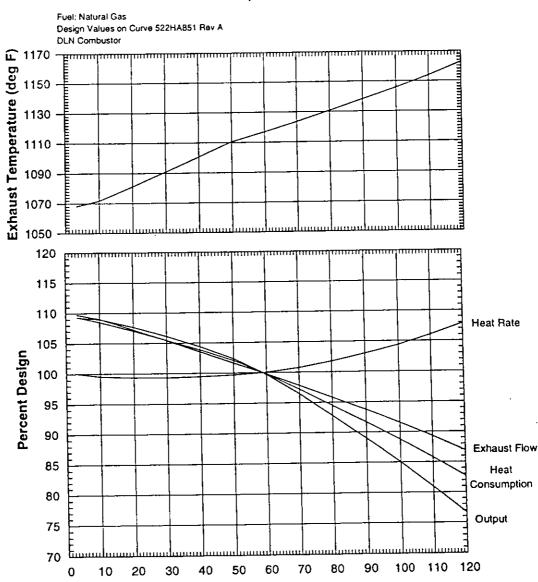
Compressor Inlet Temperature (deg F)
