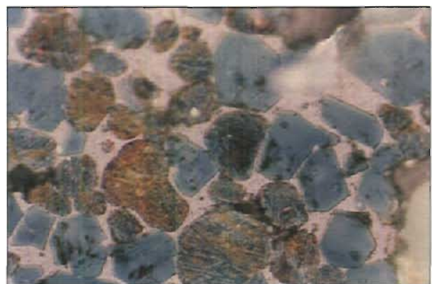
Figure 7. Polished section of clinker at 500x magnification produced with the Gyro-Therm kiln burner in operation on kiln 3. Alite crystal size and shape appear considerably improved.
