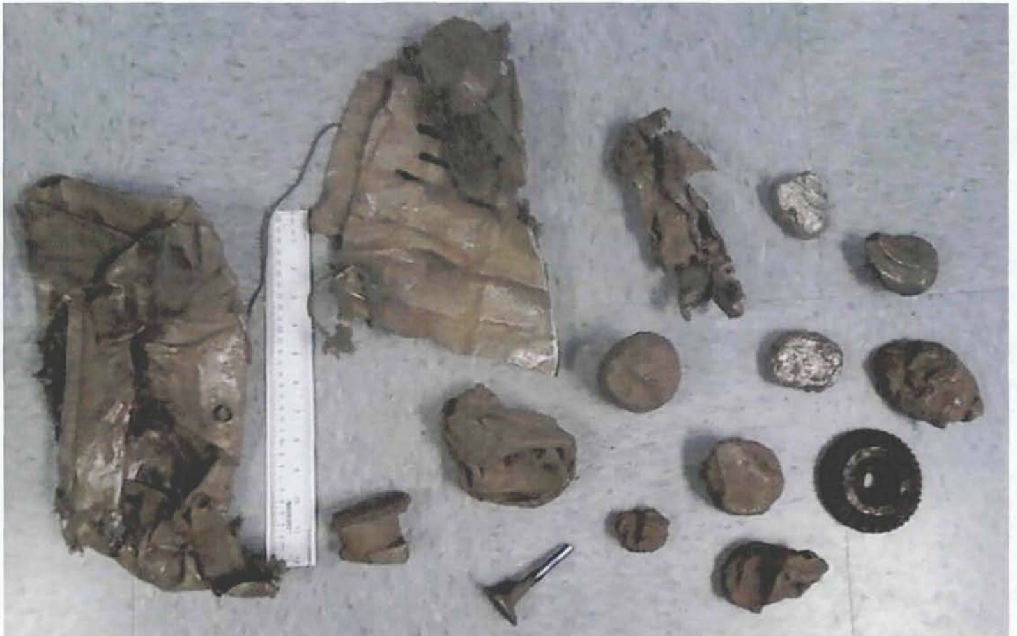
Figure 3.8 Example of pieces of metal pulled from the tripped feeding equipment. The 12 inch ruler is for reference of scale. It is not likely for any of these materials to have made it through the one inch trommel.
