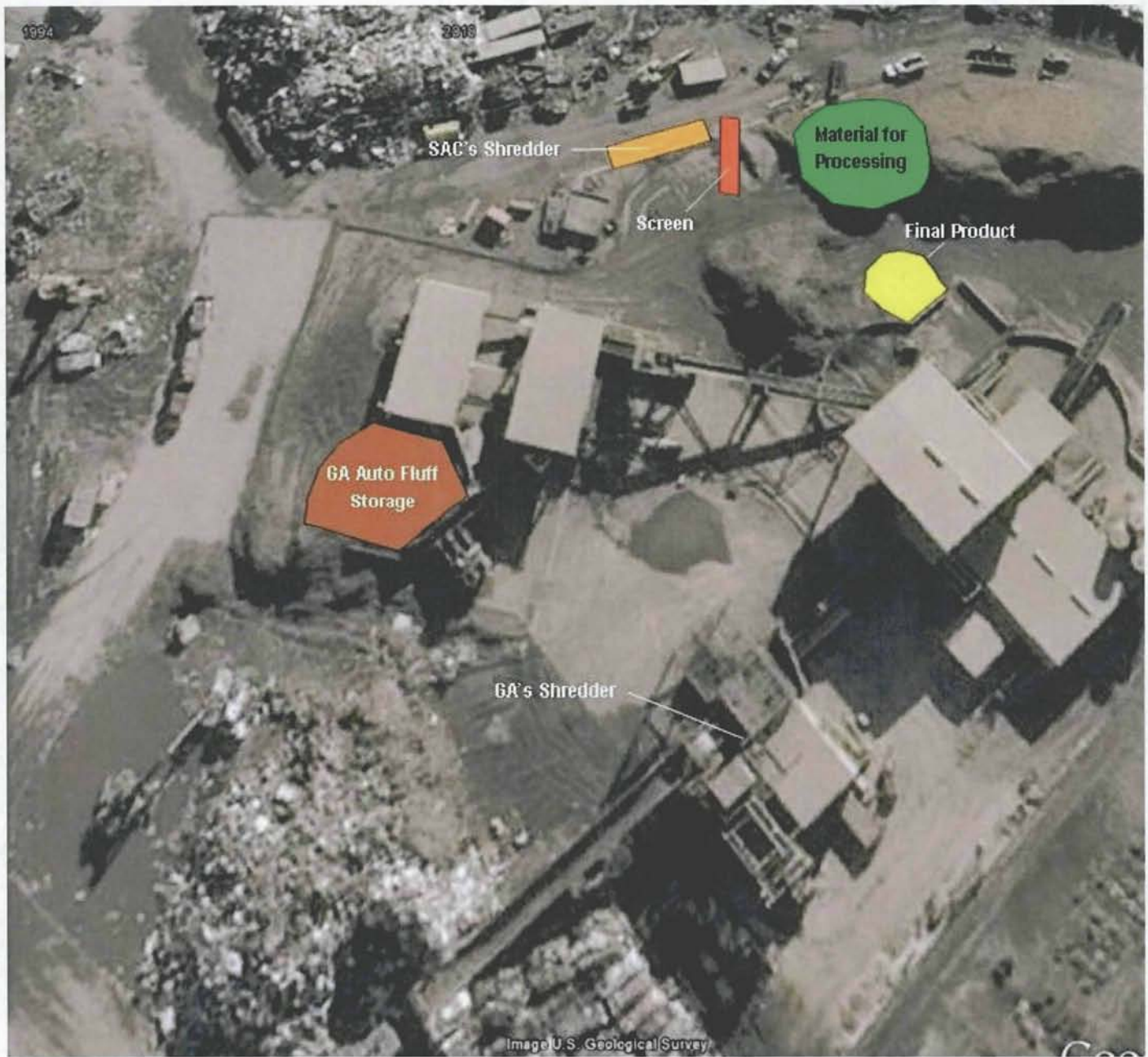
Figure 3.7 Aerial view of GA shredder operations with diagrams showing the location of SAC's re-shredding operations.
