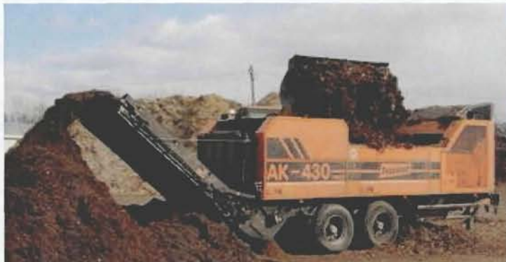
Figure 2.2 Image of a Doppstadt AK 430 in operation. The AK 630 is similar only larger.
