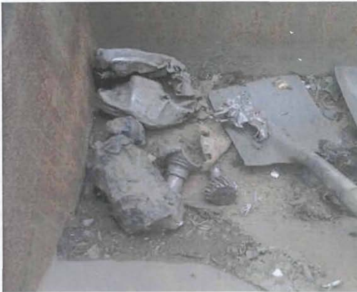
Figure 3.2 Examples of metal contamination present in the auto fluff. The shovel head is present for size comparison.
