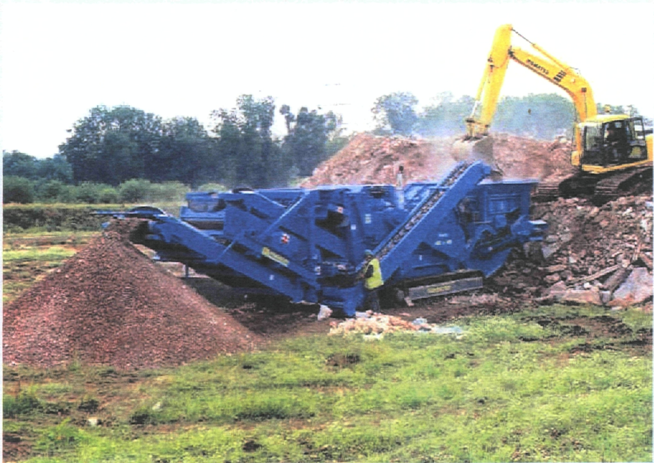
All in one Tracked Impact Crusher with Product sizing screen & re-circulation facility
