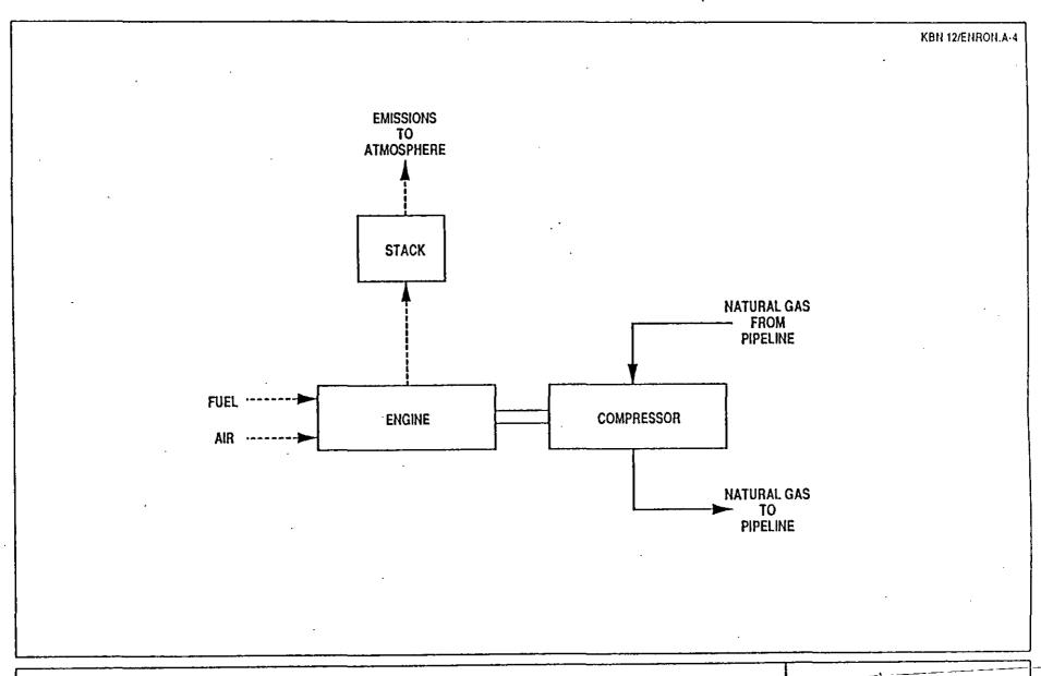
Figure 2-2 PROCESS FLOW DIAGRAM OF AN INTEGRAL ENGINE-COMPRESSOR UNIT
