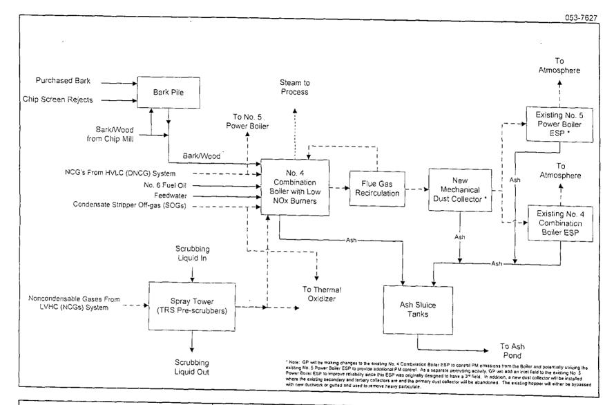
Attachment GP-EU1-I1 Process Flow Diagram No. 4 Combination Boiler Georgia-Pacific Palatka Mill Process Flow Legend
