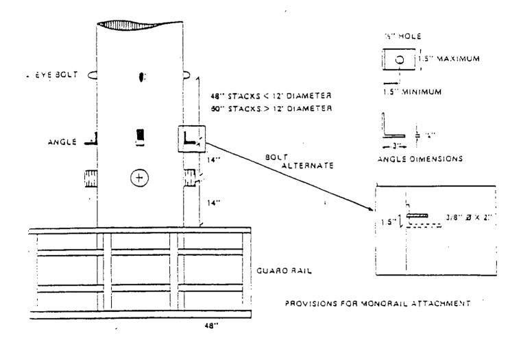
IF EYEBOLT IS MORE THAN 120 INCHES ABOVE THE PLATFORM A PIECE OF CHAIN SHOULD BE ATTACHED TO IT TO BRING THE POINT OF ATTACHMENT WITHIN SAFE REACH. THE EYEBOLT SHOULD BE CAPABLE OF SUPPORTING A 500 POUND WURKING LOAD.
