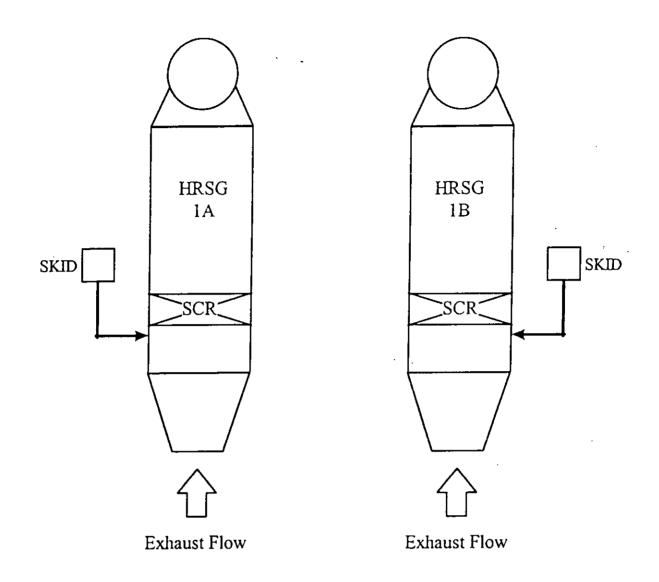
FIGURE 1 - SCR SYSTEM LAYOUT: PLAN VIEW
