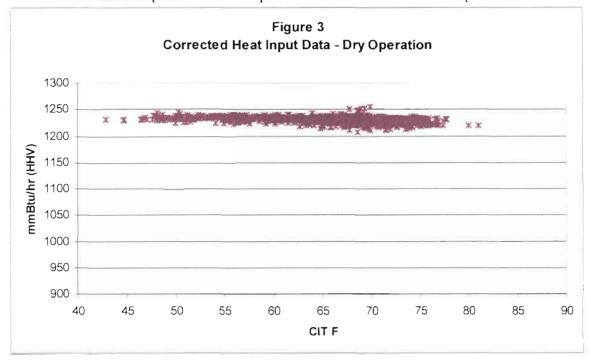
Based on the permit limit of 1214 mmBtu (LHV) at ISO conditions, APP uses this equation to check the measured data for compliance. Operation in compliance are conditions in which HIc is less than or equal to 1214 mmBtu LHV. Note that the data presented in this figure is mmBtu per hour in HHV and thus is below the equivalent HHV permit limit of 1,347.5 mmBtu/hour HHV.
