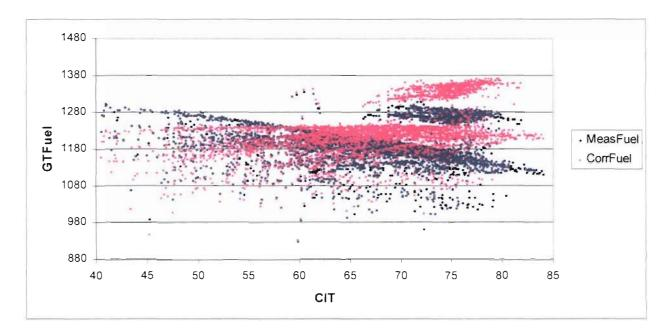
Notice that the top edge of the non-wet-compression data flattens out confirming quality of methods.
