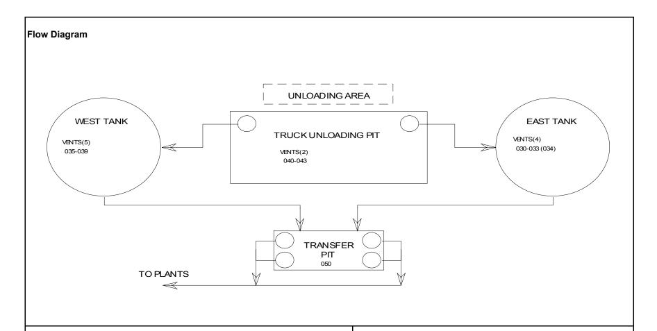
The molten sulfur handling system has no specific emission control equipment. Handling practices are specified by the Rule 62-296.411, F.A.C., Sulfur Storage and Handling Facilities.
