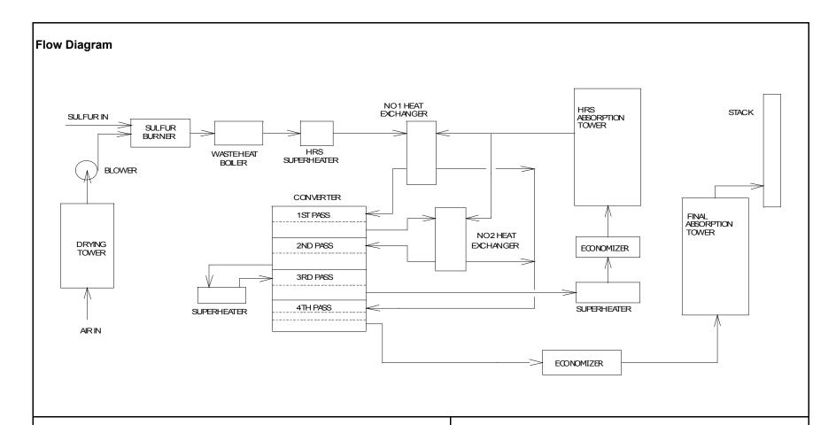
The Sulfuric Acid Plant consists of a double absorption system. Acid Mist emissions are controlled by a demister.
