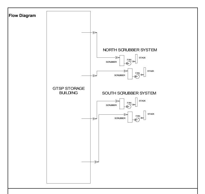
The emissions are controlled by two parallel systems each consisting of two cyclonic scrubbers and fans. Each scrubber pair vents to a common vertical stack. Each scrubber uses process water as the scrubbing liquid.
