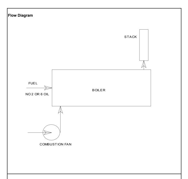
The boiler has no specific emission controls. The emissions are limited by the type of fuel oil consumed.
