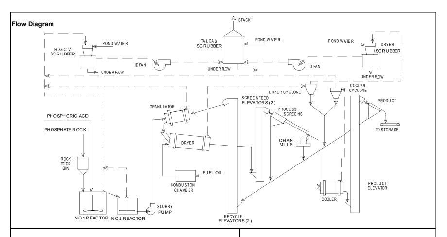
The emissions are controlled by two parallel systems each consisting of venturi scrubber followed in series by vertical 2-stage packed scrubber using process water.
