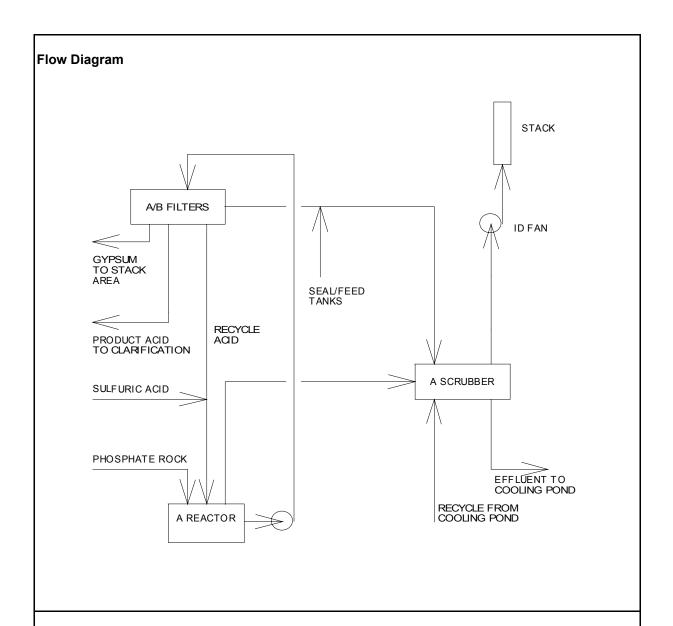
The emissions from the reactor, filter and seal tanks are controlled by a crossflow scrubber using process water. The scrubber contains Kimre Pads as its packing material.
