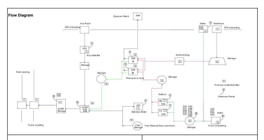
This is the overall process flow diagram for South Pierce. The emission points and emission unit ID numbers are shown.
