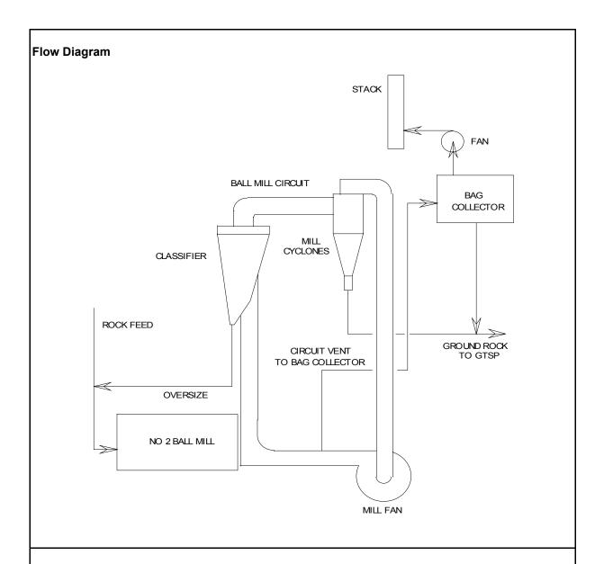
The emissions are controlled by a pulse type bag collector. It is vented by a fan located upsteam from the collector. The fan discharges to a vertical stack.
