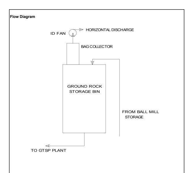
The emissions are controlled by a pulse type bag collector. It is vented by a fan located upsteam from the collector. The fan discharges horizontally.
