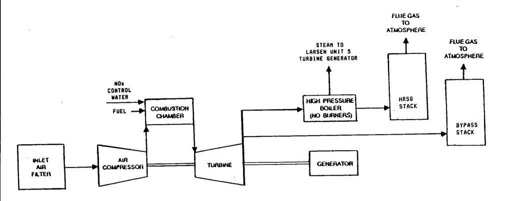
FIGURE 2-3. COMBUSTION TURBINE FLOW DIAGRAM
