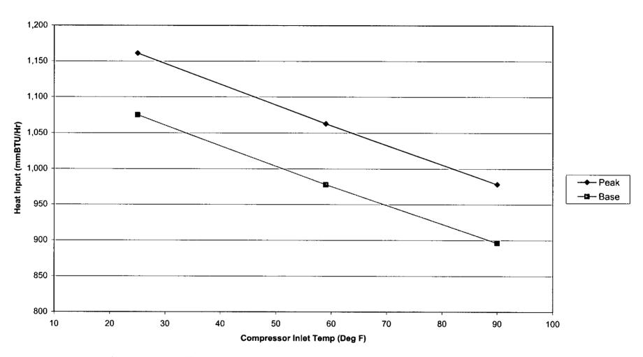
Note: Curves based on GE data for 60% relative humidity, new and clean condition. Actual performance will vary depending upon turbine inlet conditions (e.g., fogging), NOx injection water and turbine backpressure.
