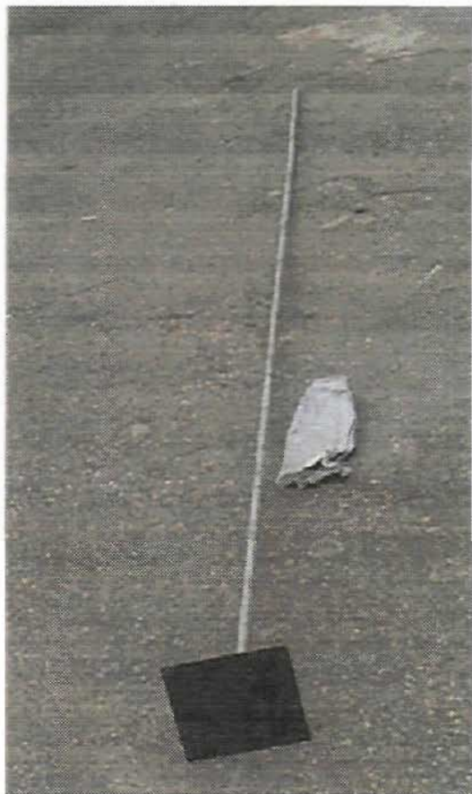
Figure 3 Measuring pole with 6-inch markings and cloth filter
