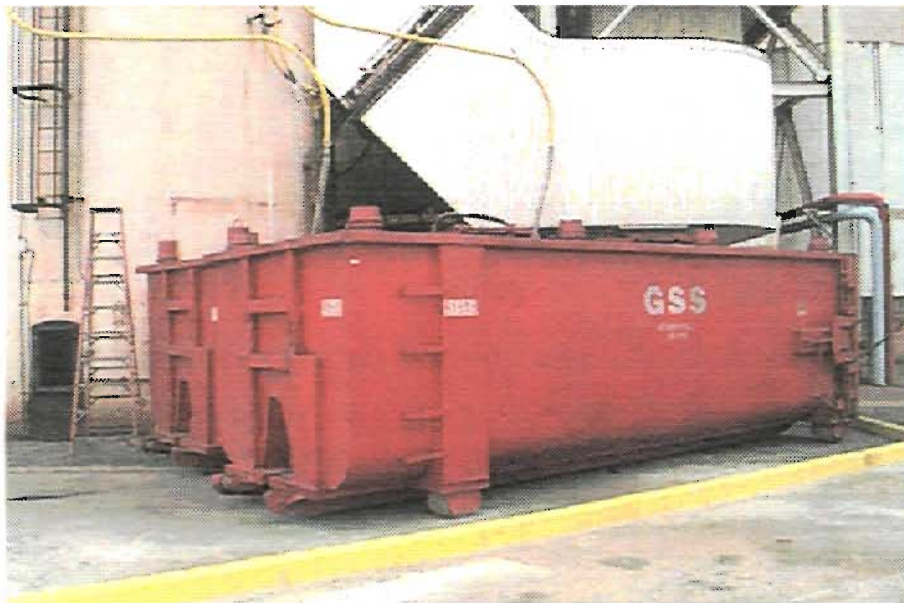
Figure 1 Transportable fly ash bins
