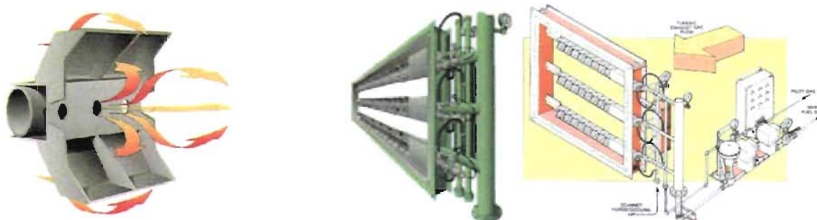
Figure 12 – Individual Burner and Array within Supplementary-Fired HRSG (Coen)
