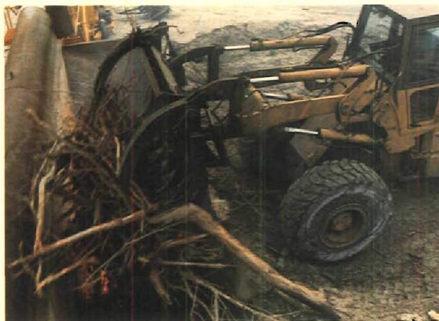
during loading, the air curtain is temporarily broken, but is quickly restored as the material drops into the burning chamber
