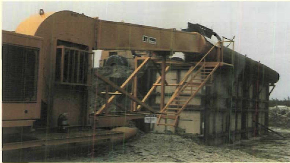
the pit shown is constructed in sections and can readily be moved and reinstalled at another location
