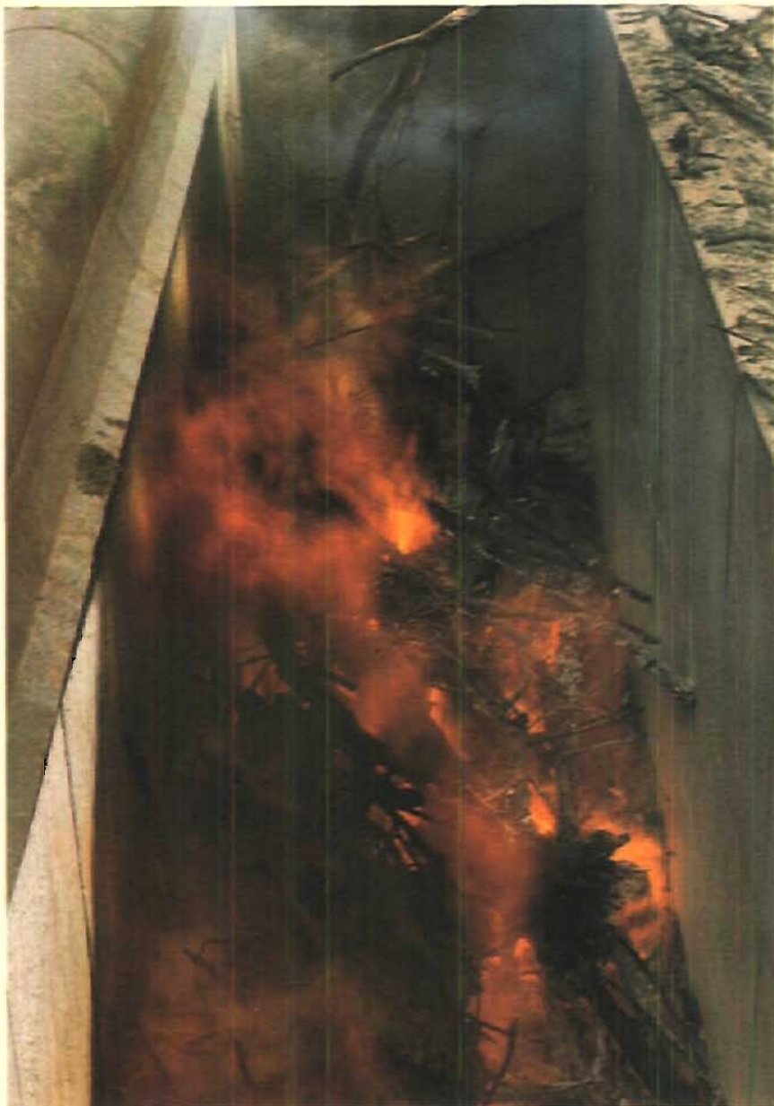
smoke is contained until complete combustion by use of both an air curtain and supplemental air supplied underneath the pit
