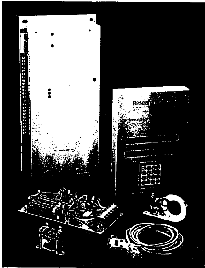
The two main components of the backfit package (for installing the MTC system into existing control cabinets) are the Interface Board (top left) and Microprocessor Module (top right). Also shown are the signal conditioning resistor panel, current transformer, potential transformer and interface cable.
