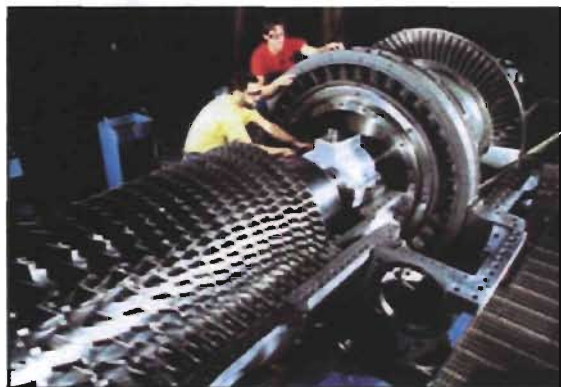
Figure 3. A GE 7FA on a half-shell Figure 4. Preassembled GE 7FA ready for shipping
