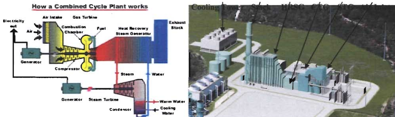
Figure 5. Components of a Combined Cycle Unit and Artist Rendition of CIPP Unit 4
