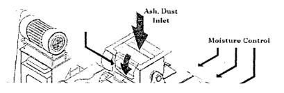
paddies, mounted on the counter-rotating shafts, blend and mix the material as it is conveyed forward. As the material is moistened by the wetting sprays, the interposing mixing paddles cause all dry surfaces to be exposed, resulting in a forced mixing and wetting of all material.
