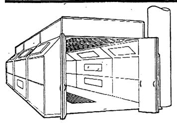
CONCEPT II is designed so that replacement air passes through filters in the ceiling and flows downward around the vehicle and into filtered gratings in the floor. This downdraft air flow pulls the overspray down into a pit instead of along the length of the vehicle as in conventional spray booths. The end result is a cleaner, factory-like finish since the chance of overspray and contaminants collecting on a freshly painted vehicle are minimized.
