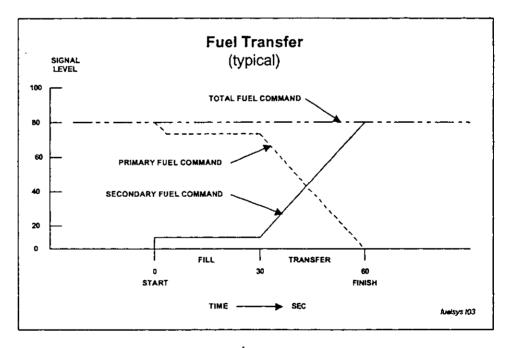
The transfer sequence is divided into two parts: a line filling period and the actual transfer. During the first period, the incoming fuel command increases to a level that will allow filling of the system in about thirty seconds, and the outgoing fuel command decreases by an equivalent amount. After fuel has reached the fuel nozzles, the incoming fuel is ramped up to equal the total fuel demand, and the outgoing fuel is ramped down to zero. Since total energy to the gas turbine is held
