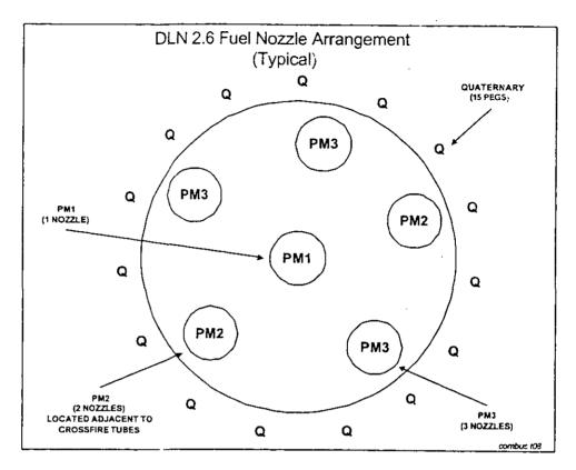
Fuel flow to the six fuel nozzles and quaternary pegs is controlled by independent control valves, each controlling flow split and unit load. The gas fuel system consists of the gas fuel stop/ratio valve, gas control valve one (PM1), gas control valve two (PM2), gas control valve three (PM3), and gas control valve four (Quat).
