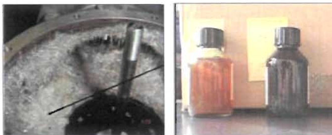
Figure 2.4 & 2.5: light tar fouls equipment & seriously contaminates condense water, Left- a gas engine control valve fouled with naphthalene crystals Right- contaminated condense water samples
