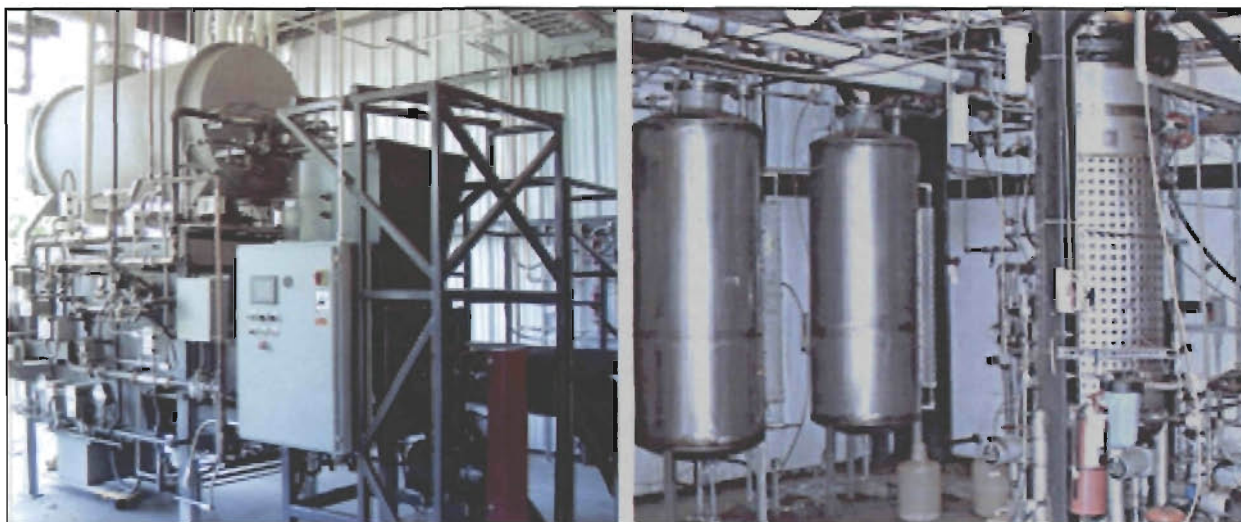
Figure 3 – Gasification System and Ethanol Production (Fermentation and Distillation).
