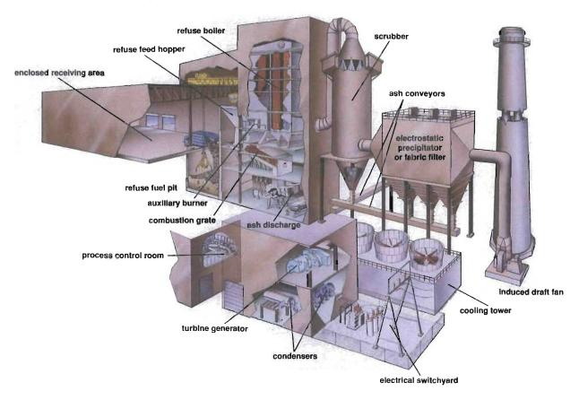
Waste is received via transfer, roll-off, or collection vehicles. Upon arrival, each vehicle is weighed at the scale house and the waste is categorized. Any unacceptable waste is diverted at this time. All acceptable waste is taken to the Refuse Receiving Building, where it is deposited onto the tipping floor or into the Refuse Storage Pit. The refuse is stored at this location until needed to charge the combustion units.
