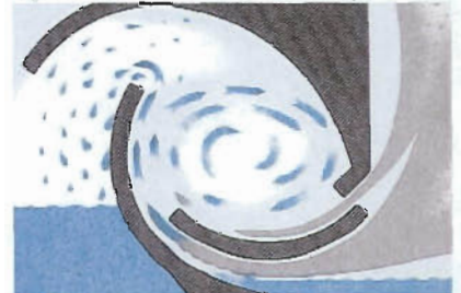
The whirl chamber performs the most critical function in a Whirl Wet's operation. This chamber causes water and particulate to combine, resulting in high-efficiency dust collection.
