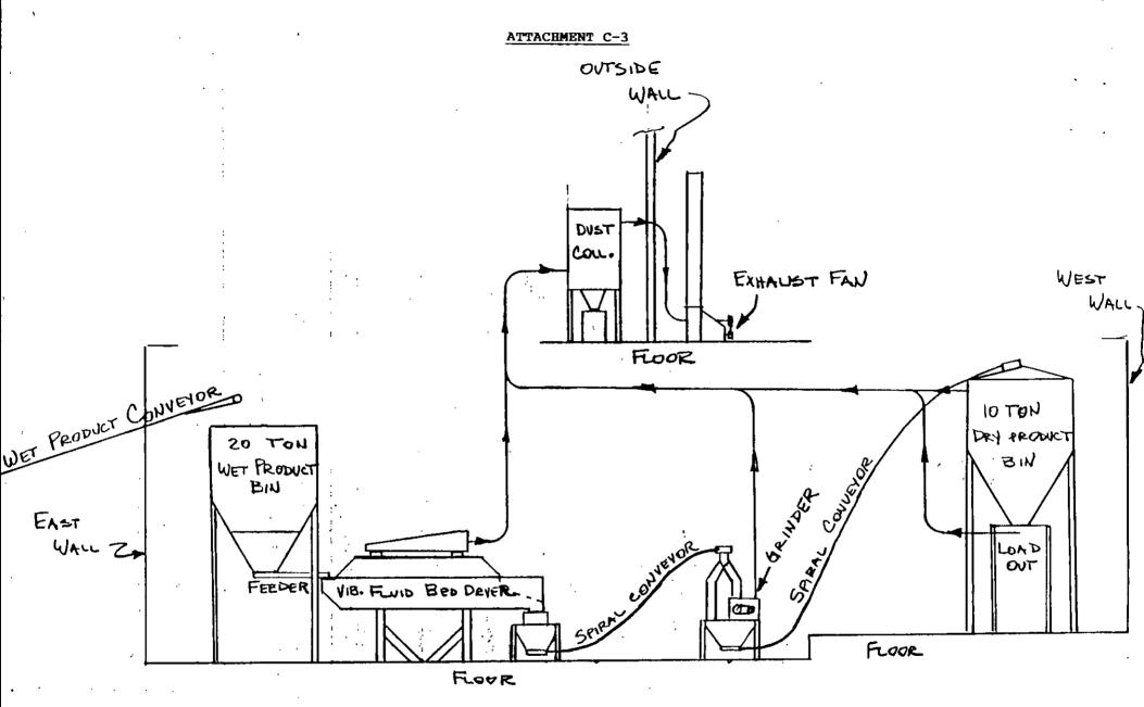
FLOW SHEET- KBF4 DRYING/GRINDING
