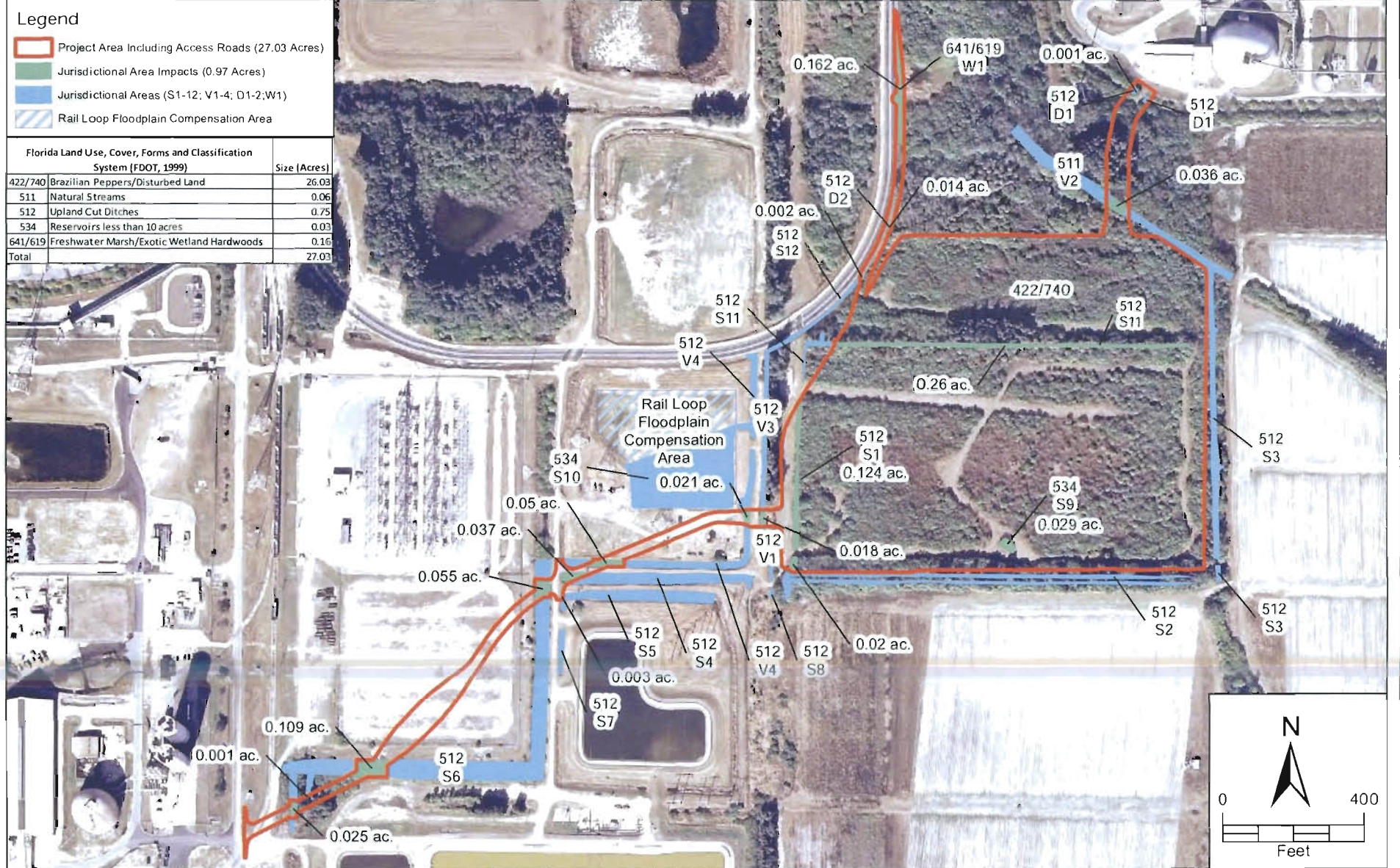
FIGURE 7. JURISDICTIONAL/LAND USE AND COVER MAP TAMPA ELECTRIC COMPANY BIG BEND POWER STATION GYPSUM STORAGE AREA/CONVEYOR IMPROVEMENTS PROJECT HILLSBOROUGH COUNTY, FLORIDA Sources: SWFWMD Aerial Photograph, 2011; Sargent & Lundy, 2011; ECT, 2012
