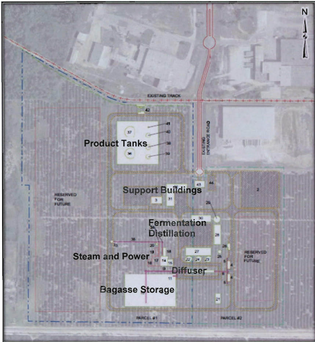
Figure 3 – Preliminary Layout of Future HEF Facility
