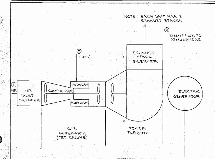
NOTE: EACH UNIT CONSISTS OF I ELECTRIC GENERATOR AND S JET ENGINES
