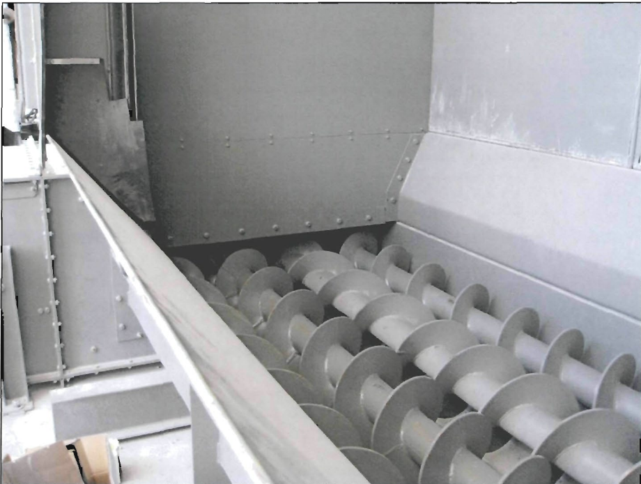
FIGURE 3. SCREW CONVEYOR IN BOTTOM OF OFFLOADING PORTS.
