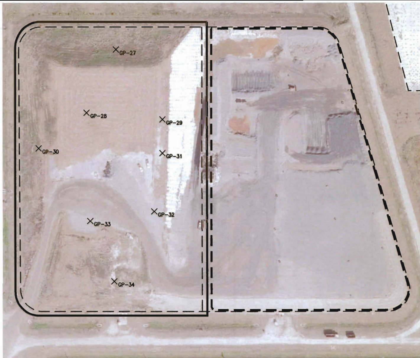
FIGURE 3 TIER 2 SAMPLING PLAN ASH MONOFILL LEE/HENDRY COUNTY REGIONAL SOLID WASTE DISPOSAL FACILITY
